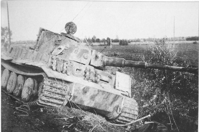
This Panzerkampfwagen VI Ausf. E Tiger I had a dark yellow base color and was camouflaged with small green and brown flecks. It had a registration number in red or blue. Many extras had been removed from the tank, such as the smoke grenade launchers on the turret and the mine launchers on the hull of the tank. One point identifies the Tigers of s.Pz Kp. Hummel. A piece of transport track was fitted to the front armor. Three links were fitted between the driver's vision slit and the front machine gun and three standard links were sometimes placed on the sides of the armor plate. Photos from Belgium and Germany also show that the unit possessed later Tiger I versions. The hull with steel wheels was sometimes combined with the old turret and some of these combinations had zimmerit, the majority not. (M. Bando)
