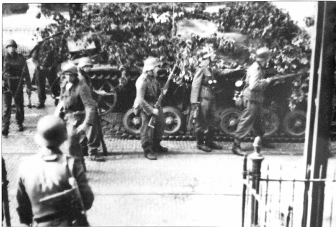
From this photo one can determine the type of StuG involved. On the roof it can be seen that the loader hatches open sideways, and this indicates that it is a later G version. The remotely operated MG that should have been on the roof is missing. (BA 497/3530/34)
