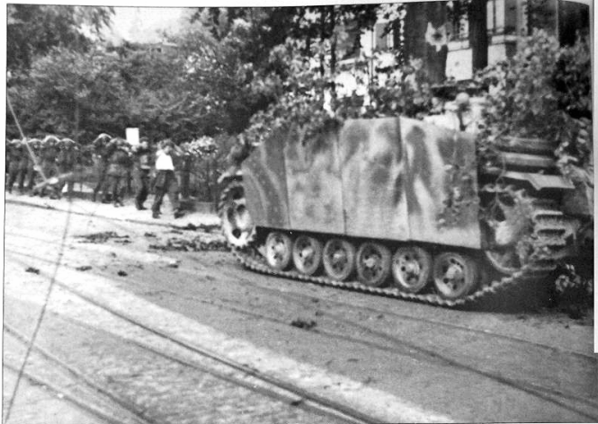
Major Kühme's Sturmgeschütz is shown here on Wednesday the 20th driving on Utrechtseweg near the crossing with Stationsweg. It is odd that on this date this SP could approach so close to the British positions, which were mainly on the west side of the crossroads. The reserve roadwheels, usually located on the engine deck, were fitted on the rear part of the mudguard. The wheels were also painted green and brown. (BA 497/3529/8)
