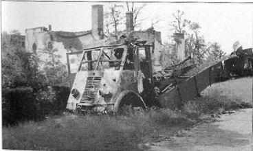
This wreck of an Lkw. 3t, Renault Typ AHN (09) with the remains of a motor-cycle in the back is seen here on the verge of the bridge ramp. It was hit by an anti-tank projectile. As with the other wrecks, this vehicle was moved to the side to clear the way for traffic, and is therefore no longer in its original position. The lorry on its side behind the Renault is an Lkw. 3t, Ford Typ S (13). (P.J. de Booy, Municipal Archives Arnhem B1620-30/5A)
