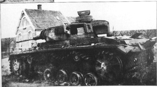
Here is the same tank, but photographed in 1945. From this picture it is clear to see that it is an old type by the old drive and tension wheel. This Panzer III Ausf. G is also shown in the photo on the Nieuwe Kade in Arnhem. This can be seen from the camouflage pattern on the front of the tank.
