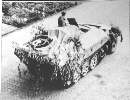
This Sd Kfz 251 Ausf. D drives through Brummen along Arnhemsestraat in the direction of Zutphen. Camouflaged with small branches and three-color camouflage, it is being driven with its engine hatches open and is loaded with spare parts including the front forks of a motor-cycle. Almost invisible but nevertheless there, hidden by the branches, is the number on the side of the hull. (Photo Brouwer-Brummen)
