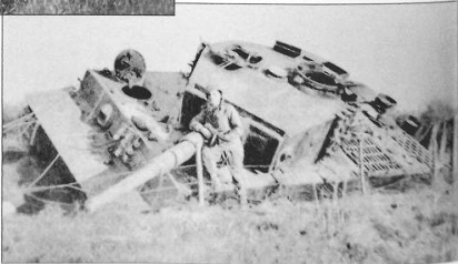
It is also clear to see that the unit possessed the older Tiger I tanks fitted with an interim type turret. This means that the commander's hatch was modified. That the chassis came from an older type Tiger can be seen from what remains of the filter system and the mine launchers on the rear deck. (Herberts Archives)
