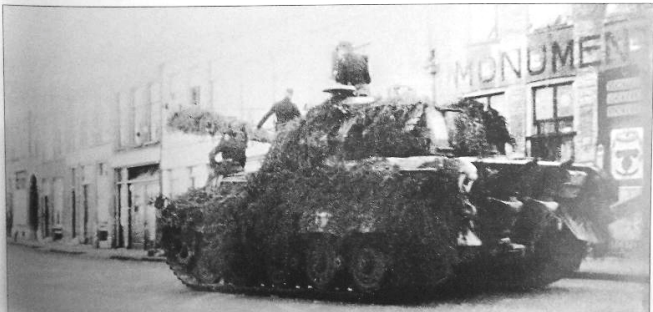
The Tiger II's were 'trained' to Aachen between 10 and 13 October. The Königstigers of 2. and 3./s Pz Kp.506 were loaded on various trains in Apeldoorn, Zutphen and Bocholt. Here one of the Tigers is being driven along Warnsveldseweg near Zutphen station. This Tiger was built before June 1944 which can be seen from the lack of armor on the hinge of the turret's rear hatch. (A.R. Schokker)
