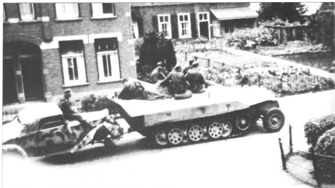
Another Sd Kfz 251 Ausf. D of SS Pz Gren Rgt 22, also driving along Arnhemsestraat and towing a Personenkraftwagen 'Pkw' Ford Type 48 1935-36 convertible. The Sd Kfz 251 is yellow overall, with no extra colors and no front mudguards. When the complete 10 SS Pz Div. had arrived in the Netherlands it was decided that all the division's armored half-tracks had to be handed over to the Recce Unit. This regiment also managed to bypass these orders because there are reports of SPWs being used by SS grenadiers of 10 SS Pz Div. These photos were taken by Mr C. Brouwer from Brummen. As a professional photographer he could not let the opportunity go by of photographing what he thought to be the permanent withdrawal of German troops. He took about 27 photos from two locations and at various times between 5 and 7 September. (Photo Brouwer-Brummen)
